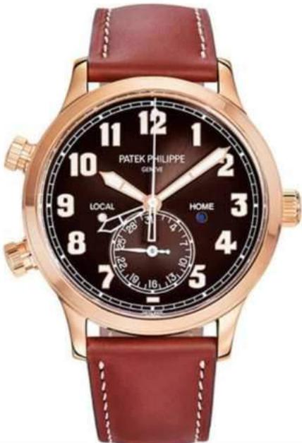
42 mm rose gold case, 10.78 mm thick, sapphire-crystal back, brown sunburst dial with black gradated, gold applied numerals with luminescent coating, caliber 324 S C FUS self-winding movement with dual time zone mechanism indicating local and home time, local and home day/night indication in apertures, local date by hand, sweep seconds hand, approximately 35-45 hours of power reserve, vintage brown calfskin strap, clevis prong buckle. Water resistant to 60 m.
